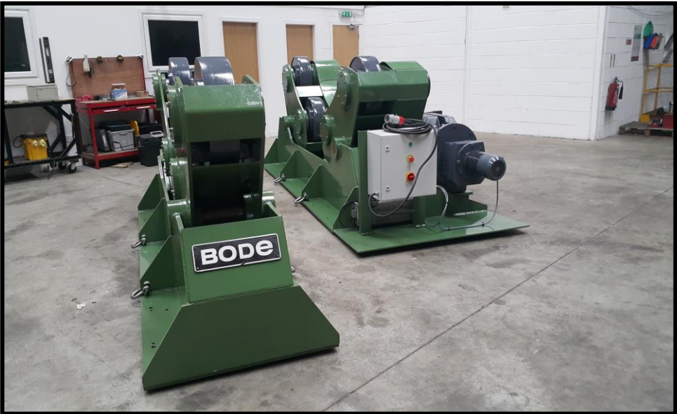
Idlers fitted with anti-creep feature
