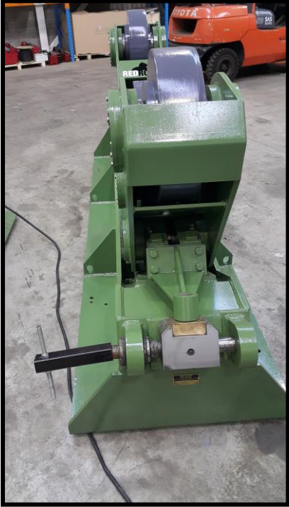
Idlers fitted with anti-creep feature
